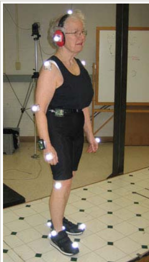
Linda Frazier, a volunteer in Lockhart's Locomotion Research Laboratory, is outfitted with motion sensors and a wrist monitor system that can detect gait instabilities that might lead to falls. Working on a National Institute on Aging-sponsored project with AFrame Digital Inc., Lockhart and graduate student Jian Liu developed the wrist monitor for tests in the locomotion lab and in nursing homes. The ultimate goal is a comfortable monitor that can alert wearers and caretakers of potential falls.
